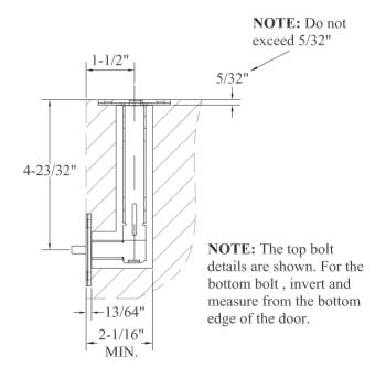
**Tip:** You can use a cylindrical latch bolt prep jig for this prep.
